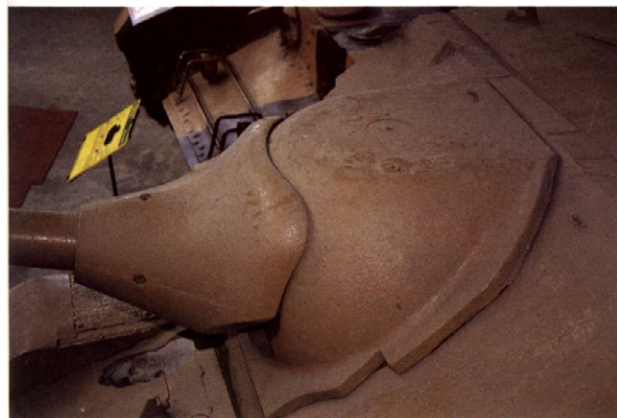
ザウコップ型鑄造防盾 Saucopf metal casting primary mantlet (right).
