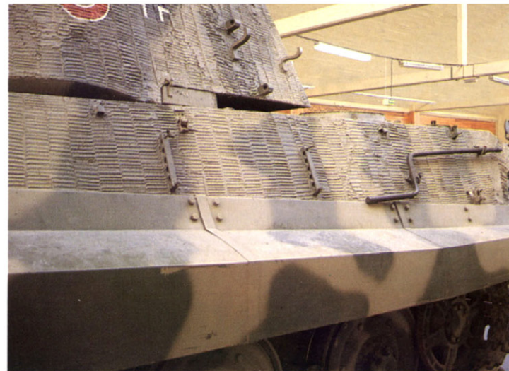
車体右側面、中央の縦長の留め金は牽引ロープと砲身清掃用の棒を留めるための物。 Right side of a hull, the brackets are for a tug rope and the gun barrel cleaning rods.
