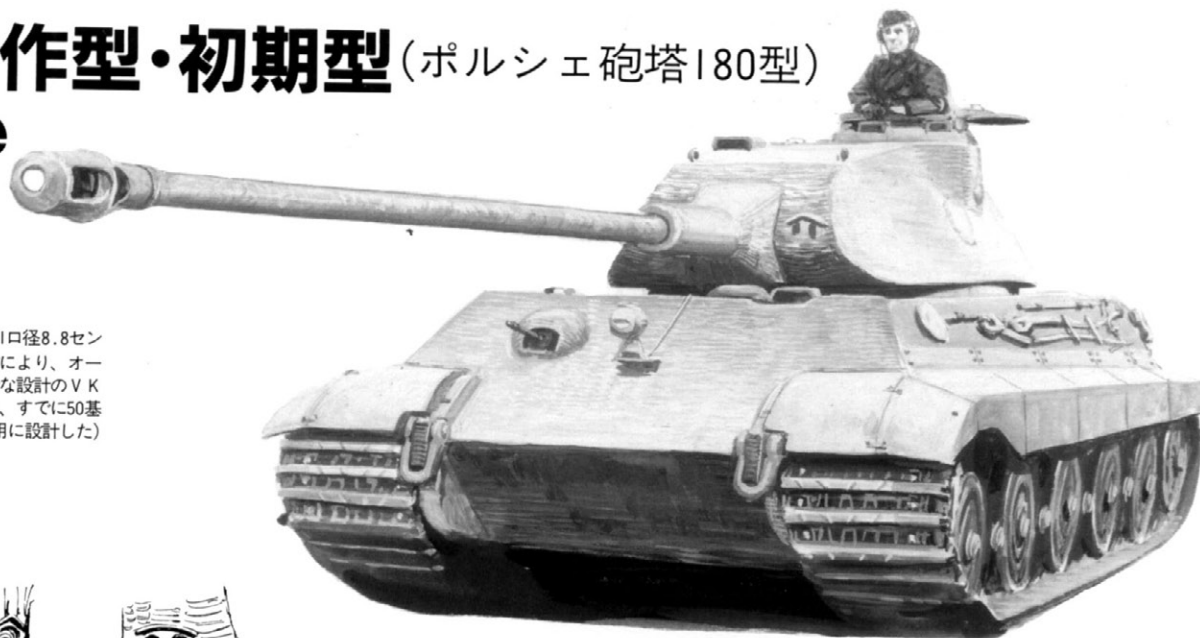
試作及び極初期型に装備された潜水装置用のシュノーケルパイプ The schnorkel pipe, was provided only on the prototype and very early production models.
