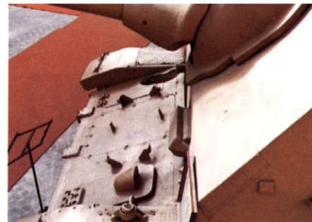
上から見た軸回転式操縦手用クラッペの形に注意。 Pivoting armoured cover for a driver's visor (top), note its shape.
