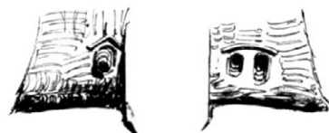
試作及び極初期型のTZF9d/1双眼式照準器孔 (右側)、試作型には雨よけのひしはつかない A couple of openings (right) for a TZF9d/1 binocular gun sight, it was found only on the prototype and very early production models.
