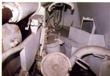
駐退管下にみえる小さな箱は砲の安全装置、右の箱は装填手用の物入れ。 The small box (under the recoil-cylinder) is a safety for the gun, a loader's kit bin is shown on its right.
