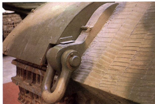
牽引フックと前部フェンダー、小さなフェンダー留め具に注意。 Frontal dust shield and towing hold with hook (right hand side). Note the small stopper for a frontal dust shield.
