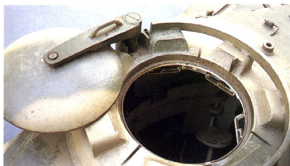
上から見たキューボラとハッチ、三箇所に刻まれた雨水抜き溝に注意。 Commander's cupola and its hatch (top), note the three notches for draining.
