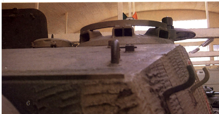
牽引フックと前部フェンダー、小さなフェンダー留め具に注意。 Frontal dust shield and towing hold with hook (right hand side). Note the small stopper for a frontal dust shield.
