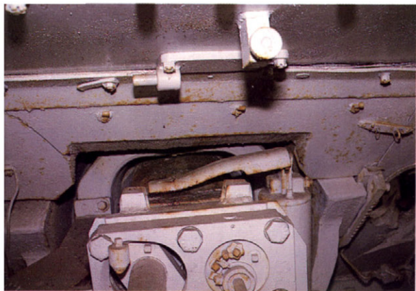
退復座器とカルダン枠上部 op part of Kardan frame, recoil buffer and recuperator housing.
