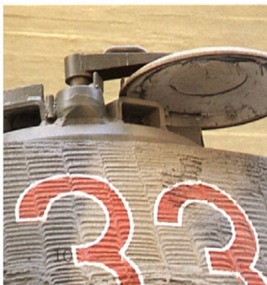
◀側面から見た車長用キューボラとハッチ。 Commander's cupola and hatch (right).
