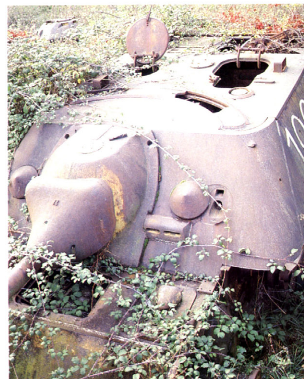
Final production type sight opening armoured traverse cover rail of panzer IV L70 (A) (the cover is missing).
